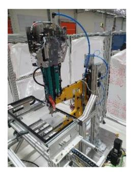
Image 01: The TOX machine tongs of type TZ (yellow) and a 50 kN strong press module (green) from TOX PRESSOTECHNIK, in combination with an XY table incl. base frame and protective fence from MiniTec, ensure process-reliable clinching of galvanized sheets for an end customer.
